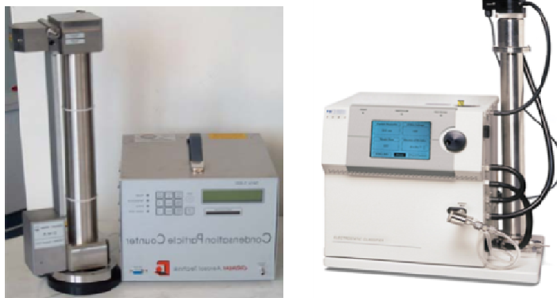
Figure 4.1 (b): Photographs of Scanning Mobility Particle Sizers used for intercomparisons
