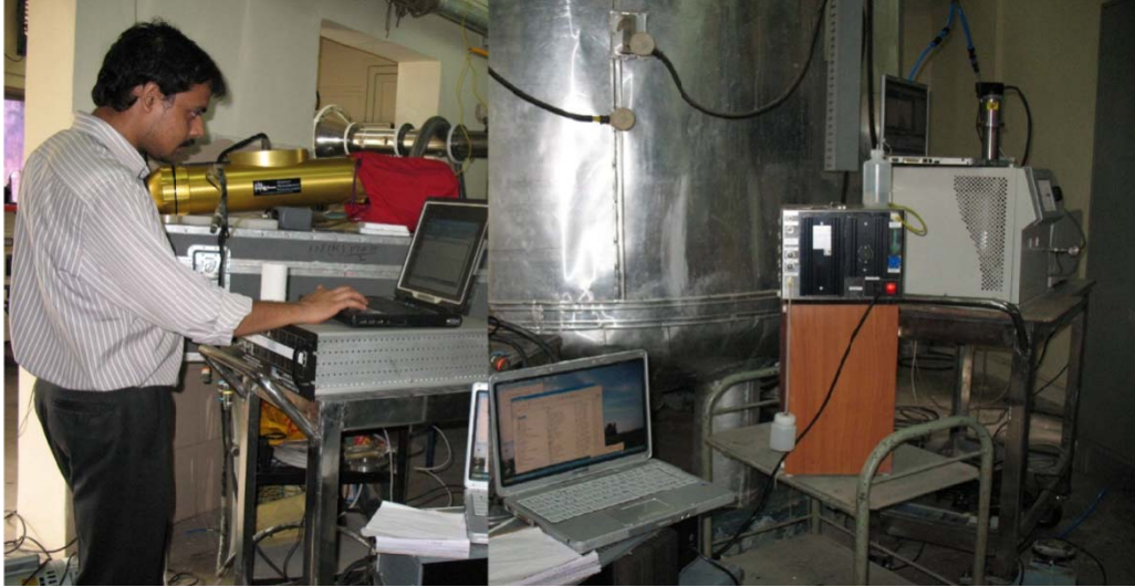
Figure 2.8: NATF test vessel and a typical set-up used for steam experiments
