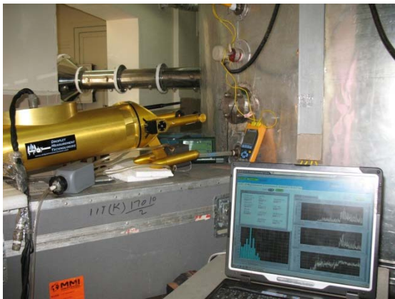
Fig 2.9 CDP sampling from test vessel
